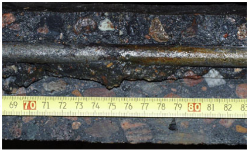
Corrosion at 75-80 cm
