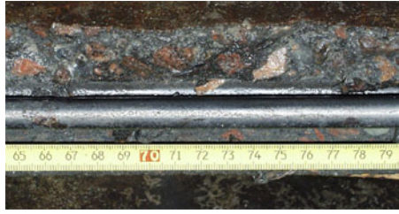
Rebar 1 Corrosion at 66, 78 cm
