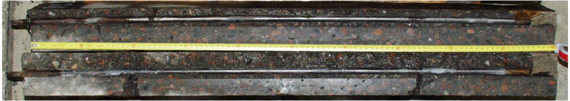
Rebars 2 & 1 Corrosion at 61, 74 cm
