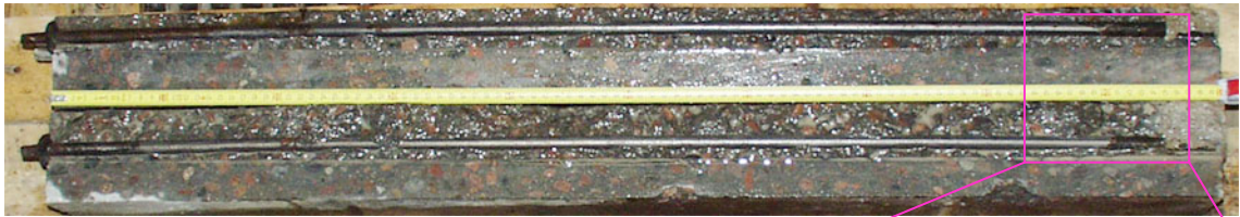
Rebars 2 & 1 Corrosion at 21, 29 cm
