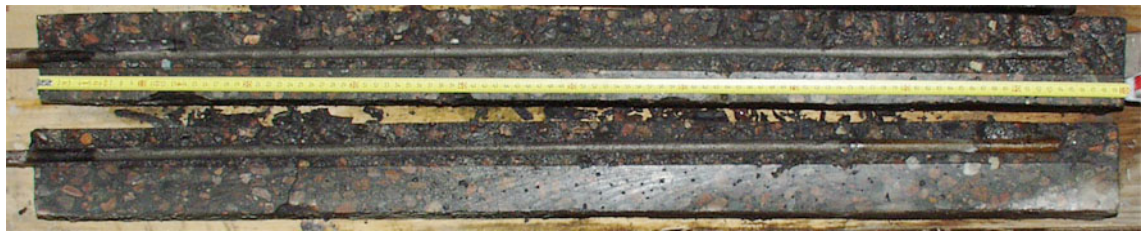
Corrosion at 75-80 cm
